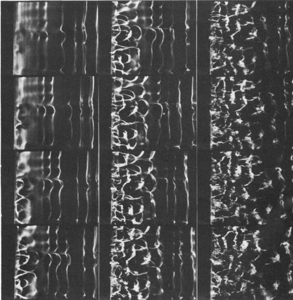
FIGURE 6. Vortex linking behind the trailing edge of the airfoil at \alpha = 20^\circ , c = 35.6 cm, R = 18250 , \Delta t = \frac{1}{64} s, t_1 = \frac{34}{84} s, h = 32 cm.
